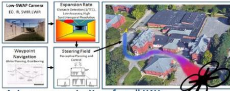
Autonomous navigation of small UAVs through complex urban environments using very low SWaP sensors and bio-inspired algorithms
